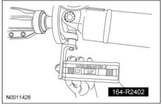
3. Using the Anglemaster II Driveline Inclinometer/Protractor, measure the slope of the connecting component. Record the measurement of the component angle as angle B.
